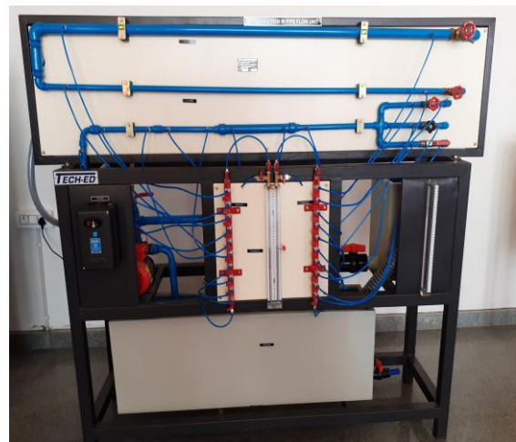
Friction in Pipe Flow
