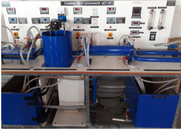
Combined Heat Exchanger Setup
