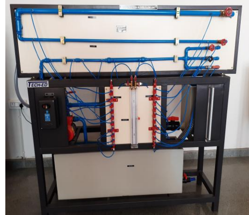
Friction in Pipe Flow
