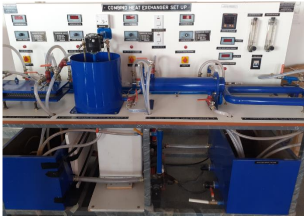
Combined Heat Exchanger Setup
