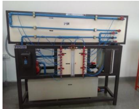
Friction in Pipe Flow
